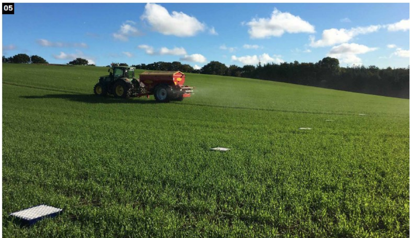
1 > A sieve to monitor grain sizes 2 > Calibration kit 3 > Measuring tube 4 > Bredal test kit The test kit includes plastic trays with dividers, measuring tube, funnel, granule strength tester and a sieve 5 > Spreading test in the field with Bredal and test trays evenly positioned.
